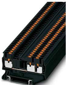
Feed-through terminal block, nom. voltage: 800 V, nominal current: 24 A, connection method: Push-in connection, 1 level, Rated cross section: 2.5 mm<sup>2</sup>, cross section: 0.14 mm<sup>2</sup> - 4 mm<sup>2</sup>, mounting type: NS 35/7,5, NS 35/15, color: black
